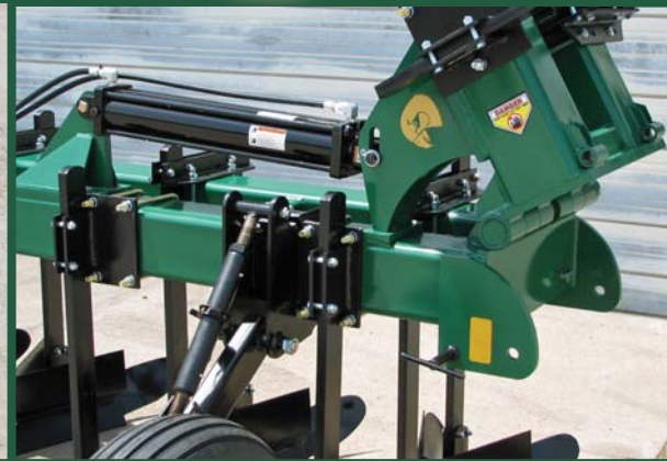
Hinged unit offers 120 degree fold & 8 degrees of float (4 up 4 down)
