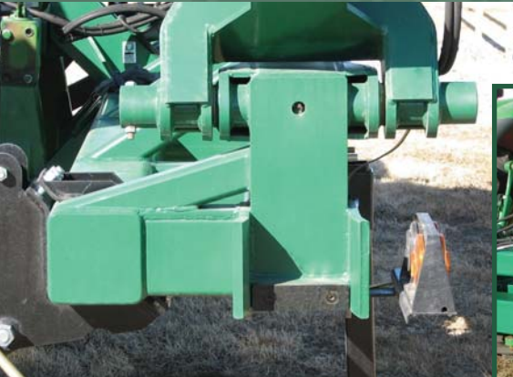
120 degrees Main Hinge in Up Position with 2 1/4" Greaseable Pin and Adjustable Wing Stop
