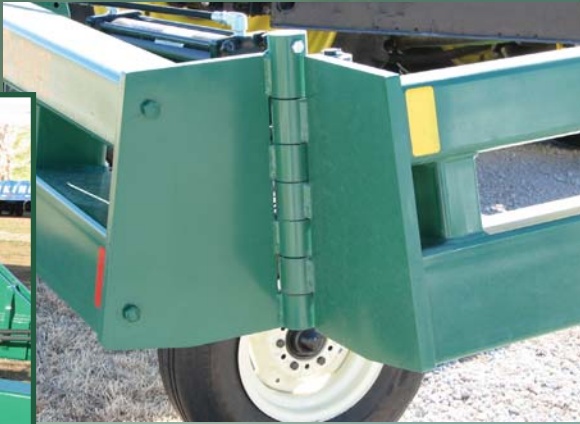
Greaseable Forward Hinge on the Double Fold Top Truss Bar
