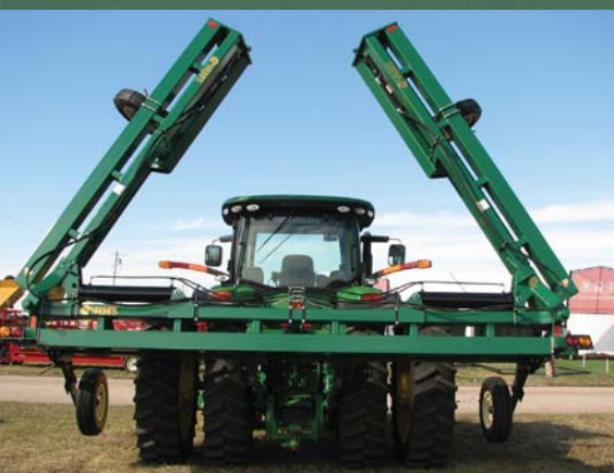
61' Top Truss Folds to 18' 2" Transport Width
