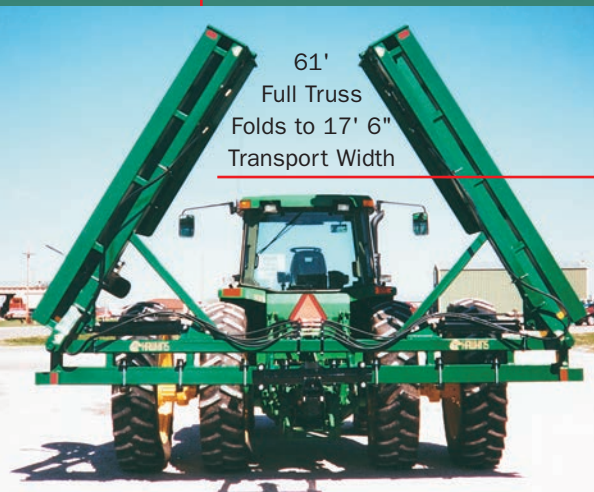
120 Degree Main Hinge in Up Position
